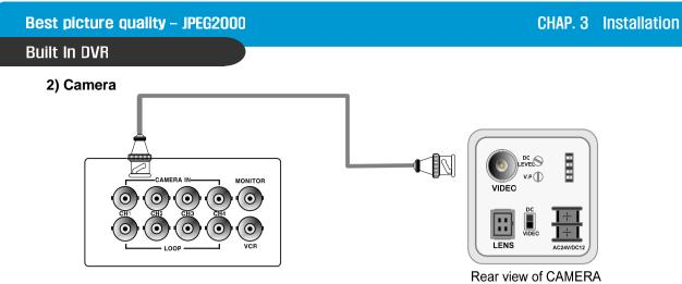
Connect cameras to the camera input on rear panel of Built in DVR.
